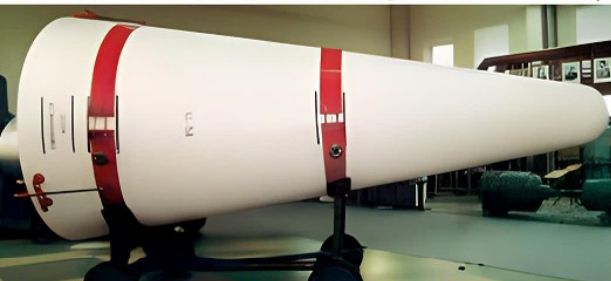
First ever Russian thermonuclear warhead for an intercontinental ballistic missile, 3 megatons yield, 8500 km range, in operation 1960 to 1966.
